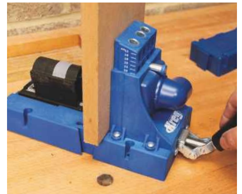
▲ This large cam lever locks the work firmly in position
